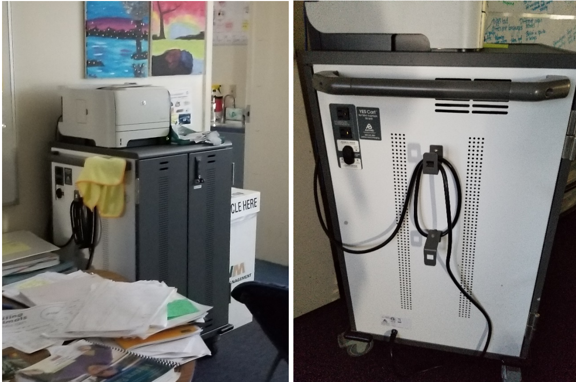
Figure 5. Multiple computer charging stations were left plugged in and operating. These units use about $0.10 – 0.25 daily per unit, which can add up when there are hundreds throughout the District. Additionally, leaving laptops plugged in for extended periods can shorten battery life.
